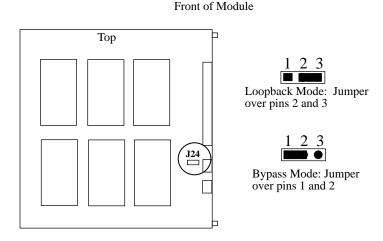
Figure 2-2 Network Bypass Jumper
